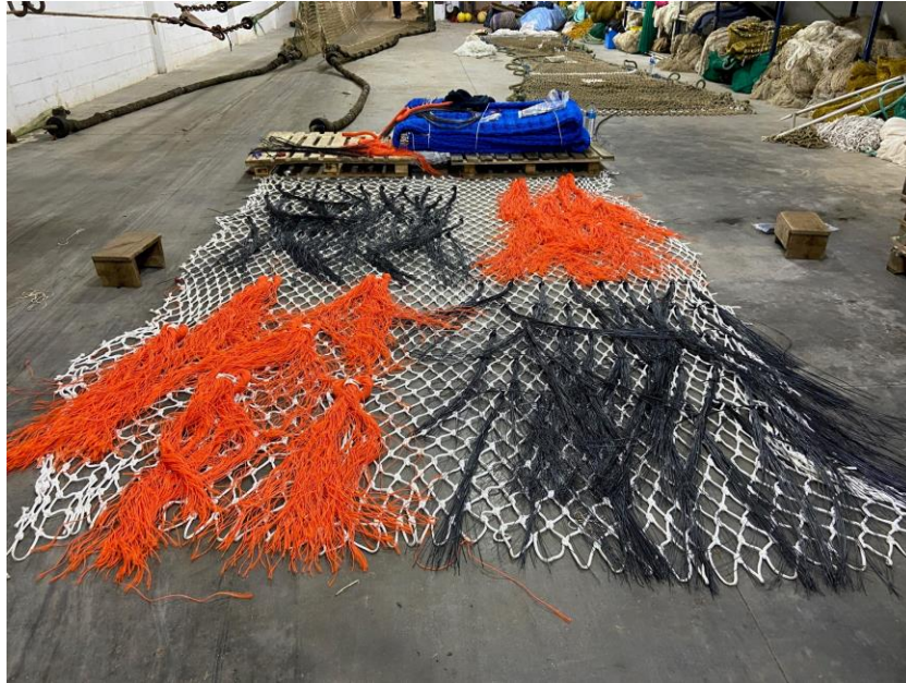
Figure 9. Trawling net arrangement to test the circular dolly ropes (black) against the conventional material (orange).
