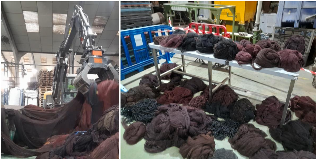
Figure 20. Opening process for the ropes, stakes and nets
