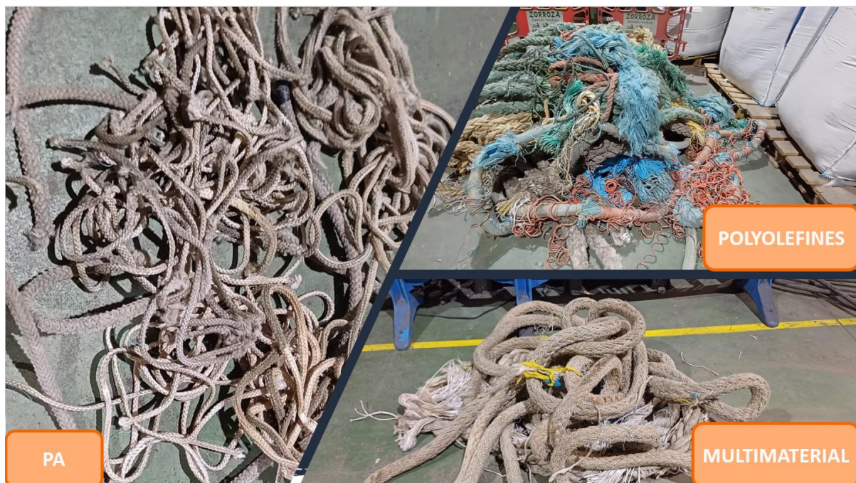
Figure 24. Materials classified and separated by composition in different groups
