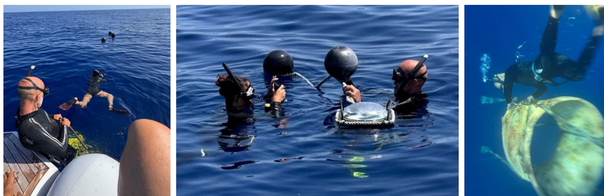
Figure 45. FAD inspection in the Mediterranean testing. Left - Retrieving the FAD to inspect the main rope. Found in perfect condition both at the surface and at the deepest section of the FAD; middle - floats found in perfect condition for the two jelly-FADs visited with this type of flotation, right - floats found in perfect condition for the three jelly-FADs visited (photos credit: ISSF by Gala Moreno):
