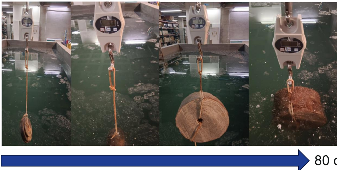
Figure 44. Evaluation of the buoyancy of Paulownia wood in the laboratory. Testing period of 80 days.
