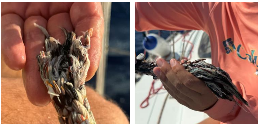
Figure 46. Breakages of 12mm cotton ropes
