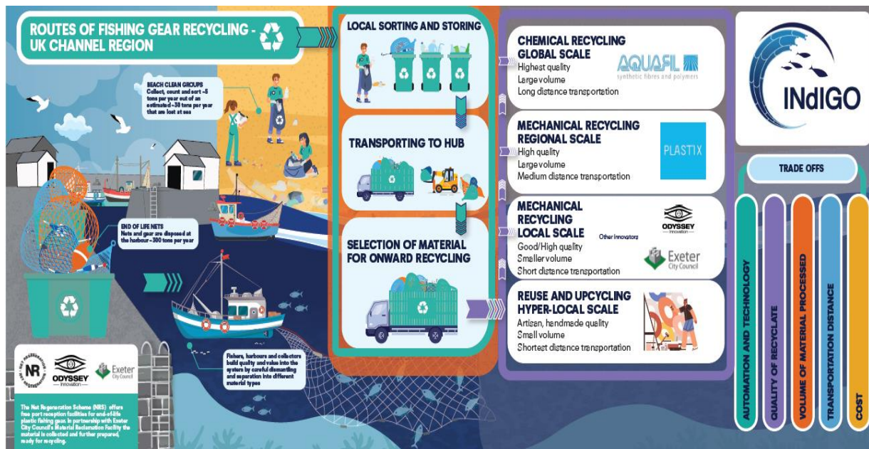
Figure 20. Current key recycling methods and their benefits and challenges for EOL FG's. 38
